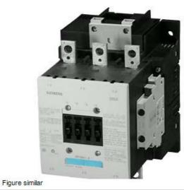
CONTACTOR, 75KW/400V/AC-3, AC(40...60HZ)/DC OPERATION UC 220...240V AUXIL. CONTACTS 2NO+2NC 3-POLE, SIZE S6 BAR CONNECTIONS CONVENTIONAL OPERATING MECHAN. SCREW TERMINAL
